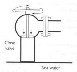
the ship. You need to close this so that you can you can cut off the pressure to the piping. If the ship is in dock for any amount of time, they should have closed the valve already. But we have boarded ships and found the valve left open. We have had to shut the valve, do our work, and then reopen the valve to sink the ship.
