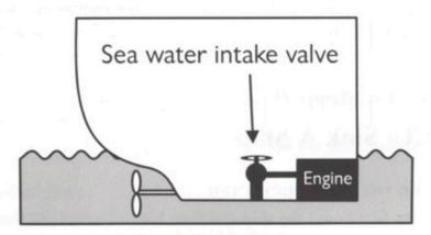
The sea water intake typically is at the bottom of the ship, but it can be on the side.
