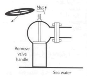
The valve handle may look either like a steering wheel or a lever type handle. Take it off. You will probably have to remove a retaining bolt that is holding the handle on. Do it and then pull the handle off. Hide the handle somewhere away from the valve stem. When you are done, we should just have a valve stem protruding outward from the valve.
